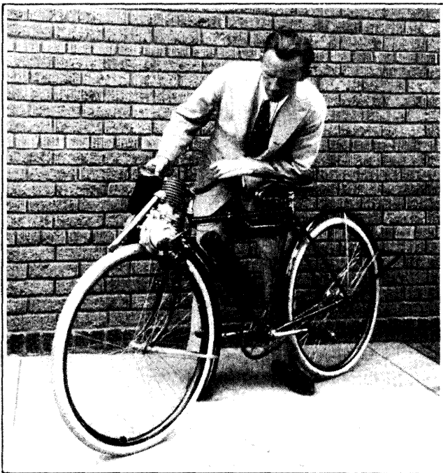
First Picture Published of Okay Motor Fitted to Bicycle. Note Compactness of Outfit Which Scales 16 Pounds. A. L. Woodruff Is Riding This Machine Through the West
