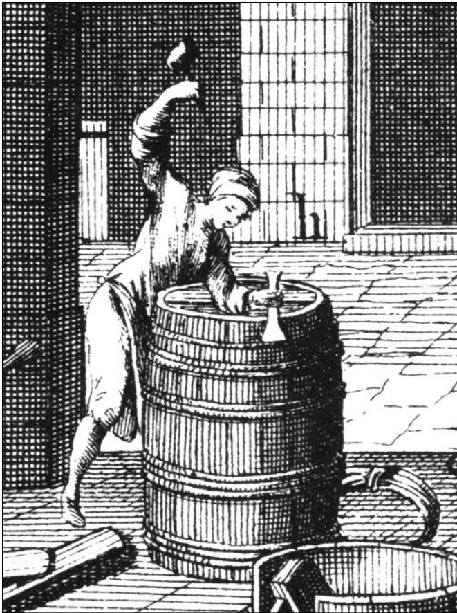
Figure 16.6. Cooper driving a wooden hoop onto a barrel, from an eighteenth-century encyclopedia. (Gillespie 1987).
